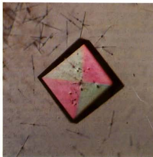
Fig. 1. The tetragonal crystal form T in a plastic dish viewed exactly along the fourfold axis under the polarizing microscope where no birefringence should be expected. Still, the two pairs of opposite triangles change colors differently upon rotation. Under glass, the whole crystal is uniformly dark at 0 and 90° rotation and uniformly bright at 45°. At angles between these positions, the pairs of opposite triangles show different brightnesses (different colors under plastic). All faces of the crystals are optically flat, i.e. there is no pyramidal growth.
